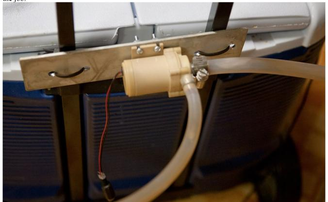
I mounted the pump on a piece of aluminum and attach it to the cooler with tie wraps. I cut the tie wraps when I want to use it on the stock pot.
