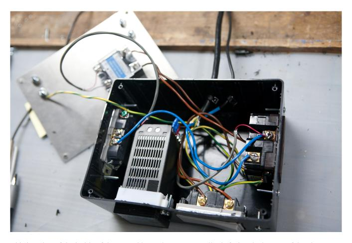
This is a shot of the inside of the control box. The PID Controller is facing the bottom of the picture, The on/off switch is next to it, the Solid State Relay is behind the box mounted on a metal cover that is the bottom of the box.
