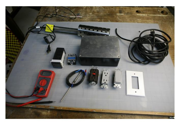
Here are all the parts of the controller. The 16AWG power cord was taken from a dead appliance. It is good to have a multimeter handy to check your wiring before you connect the power and heater and pump.
