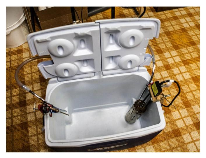
This is the front of the cooler with the supply and return lines in place in the cooler. The notches in the cover allow the covers to be closed to minimize heat loss. Another item to do will be to fill the hollow spaces in the covers with foam since they tend to collect a small amount of condensation during long cooking periods. I have not found that there is any appreciable water loss during 72 hours cooking periods and the temperature is stable at all times.
