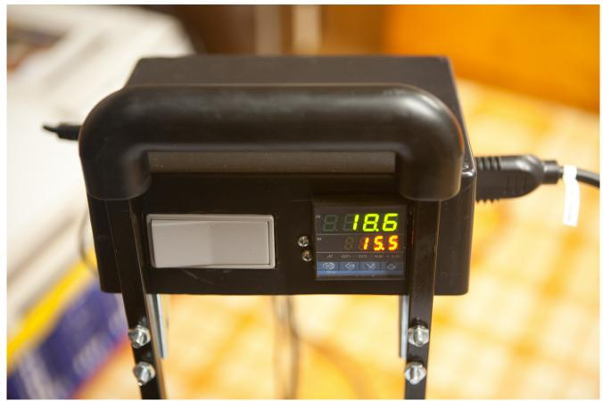
This picture shows the front of the box with the on/off switch and the PID. The box is mounted on the handle of the cooler that serves as the water reservoir in this installation. The box can be removed from the handle and placed on the counter up to 6 feet from the heater. The thermocouple lead is also 6' long so that is the maximum distance for this setup. Longer leads can be ordered if you wanted to have the box further away from the water bath.
