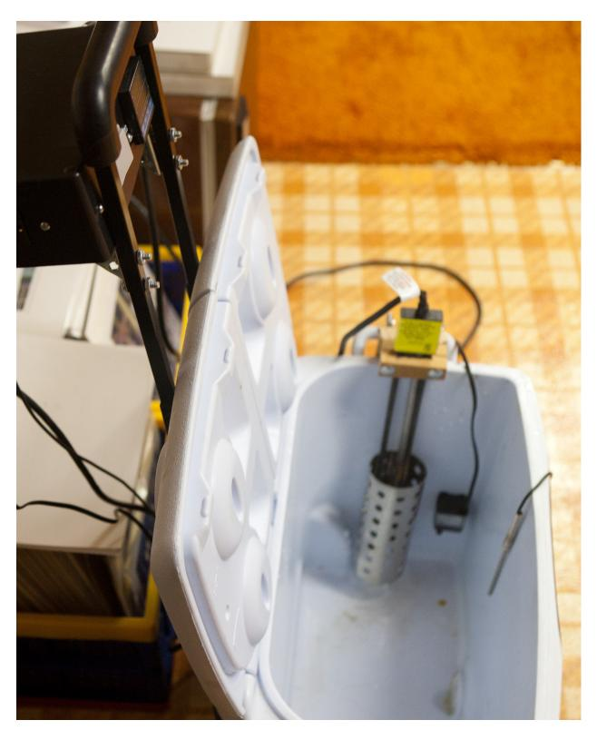
This shot shows the heater, thermocouple and pump all installed in the cooler. The wooden blocks that are holding the heater in place are a loose fit to allow the heater to be installed in different sized containers. The only rule is that the heater element must always be covered with water.
